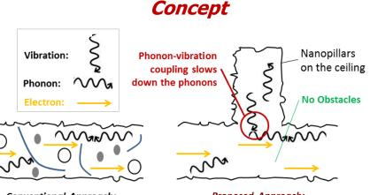
Conventional Approach: Thermal Conductivity Reduction using Scattering Obstacles Proposed Approach: Thermal Conductivity Reduction by Resonance Hybridizations
