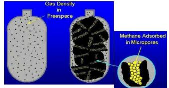
Without adsorbent With adsorbent
