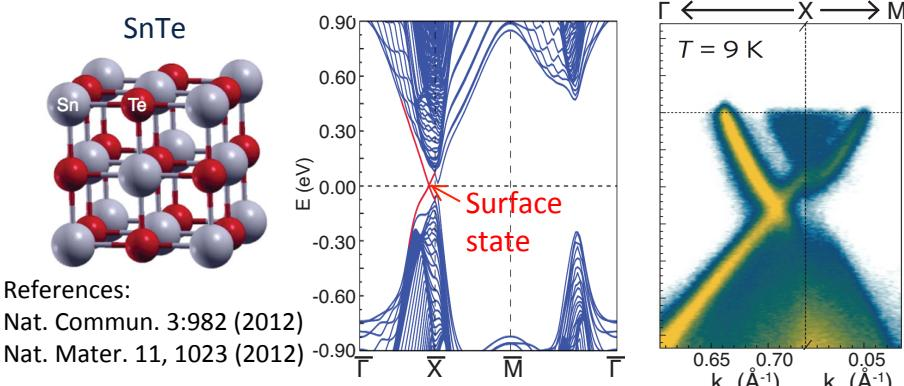
In-doped SnTe nanoplates reveal surface states.
