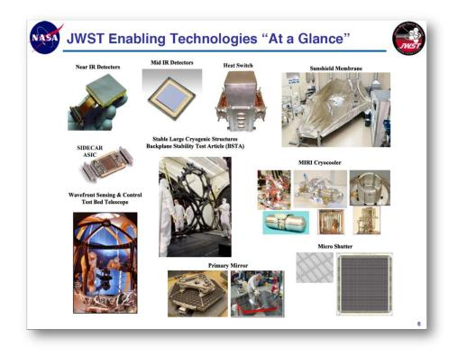
Figure 2: James Webb Space Telescope Technology Development items identified at the start of the flight program. All of the items completed TRL 6 development by 2007. Image credit: NASA/GSFC.
