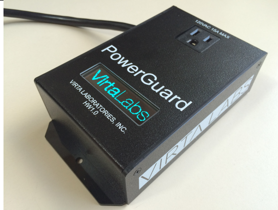
Figure 6: A smart power outlet designed to detect anomalies and malware via the AC power outlet rather than software. The power outlet uses (among other things) advanced machine learning algorithms and spectral analysis to detect unusual behavior. One can learn about basics of power analysis from an earlier research paper [2]. Photo copyright Virta Labs, Inc. Used with permission.
