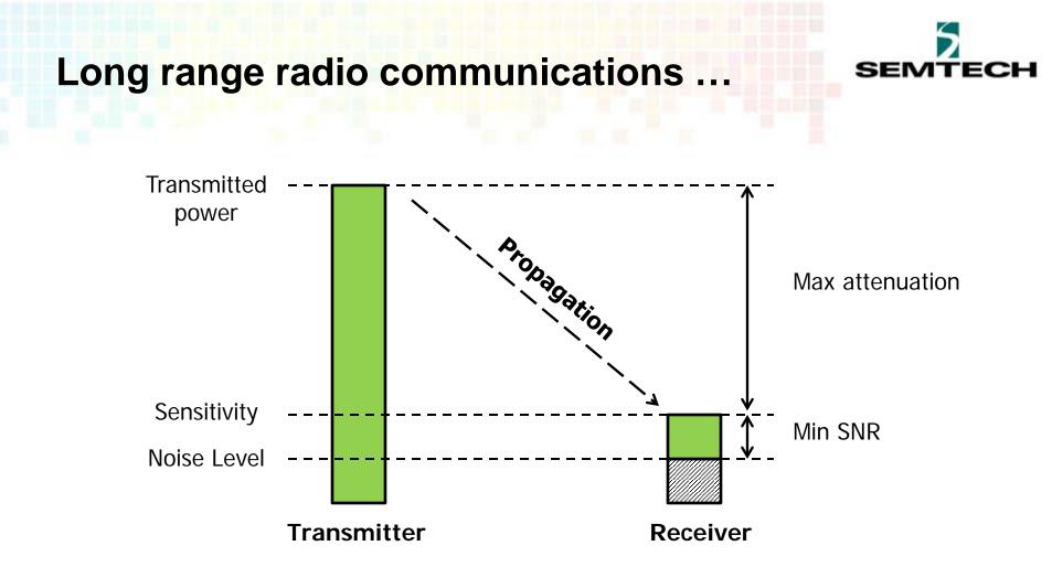
Radio range is a (vague) function of the maximum signal attenuation (or Path Loss) tolerated by the communication system.
