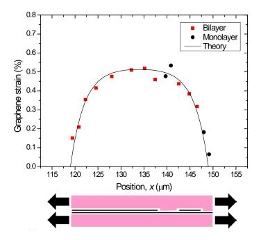
Figure 1: The strain along a graphene reinforcement in a composite measured using Raman spectroscopy. The composite has a global strain of 0.6 % and the strain in the graphene reinforcement is found to follow shear lag theory typically used for conventional macroscale fibres.
