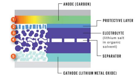
Predominant lithium ion battery separators are made from polyolefins, either polypropylene or polyethylene. These materials undergo catastrophic shrinkage above 120 C, which leads to shorting in cells that can cause the sparks that will ignite the electrolyte and flammable gasses. Several methods have been proposed to improve the thermal stability of separators, which include:
