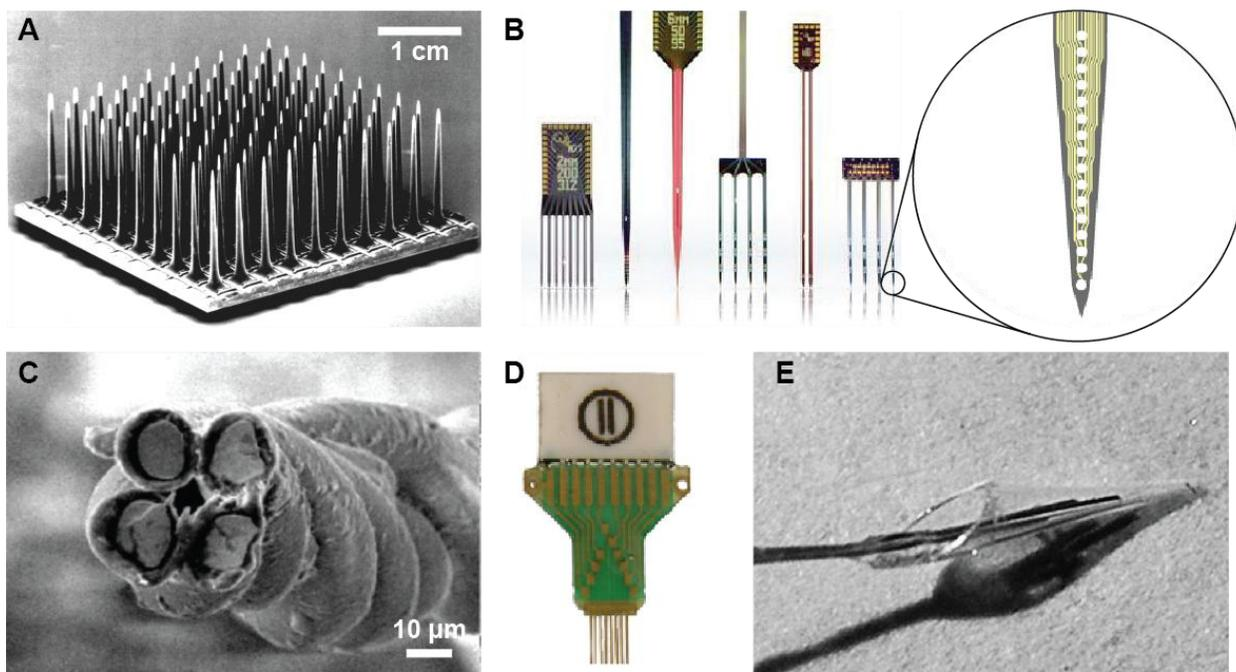
**Figure 1.** Examples of single unit and LFP recording devices commonly used in research setting. (A) Silicon multielectrode array (Blackrock Inc.). (B) Silicon multitrode probes (Neuronexus Inc.) Inset shows the detailed structure of the recording electrodes. (C) Tetraode microwire bundle (University of Queensland). (D) Tungsten microwire array (Tucker-Davis Technologies Inc.) (E) Silica cone electrode (Neural Signals Inc.)
