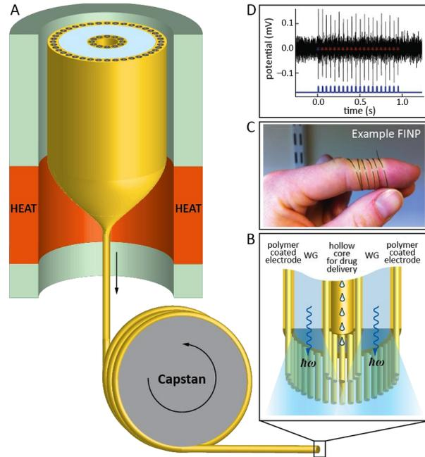
**Figure 4.** (A) Thermal drawing process (TDP) applied to FINP fabrication. (B) Longitudinal cross section of an example FINP for recording, optical stimulation and drug delivery. (C) Example FINP. (D) Optically-evoked action potentials recorded with a FINP in the medial prefrontal cortex of a transgenic Thy1-ChR2-YFP mouse expressing ChR2 in a broad neuronal population.
