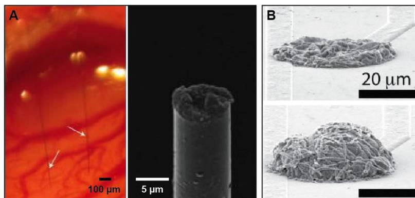
**Figure 3.** Examples of polymer and organic/inorganic composite neural recording electrodes. (A) Carbon-composite microelectrodes CVD-coated with polyxylene. Tip is electrochemically coated with PEDOT (Kozai 2012). (B) Electrodes coated with electrochemically deposited polypyrrole nanotubes (Abidian 2010).
