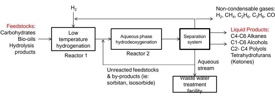
Reactor 1 catalysts: High rate of C=O Hydrogenation
