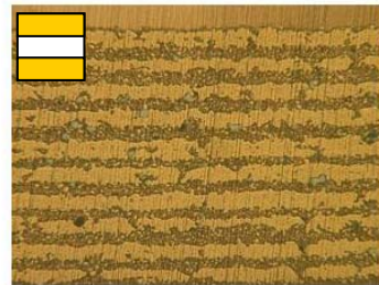
Incomplete sintered, layered structure
