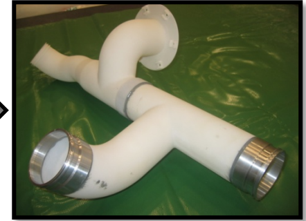
AM: 2-piece bonded assembly
