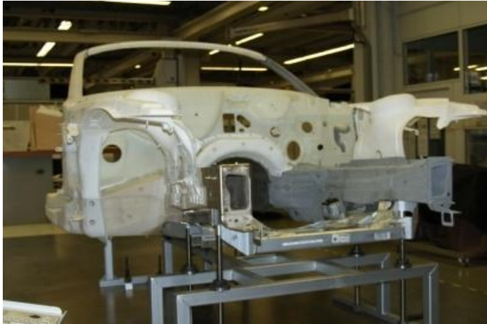
Vehicle front using SLS
