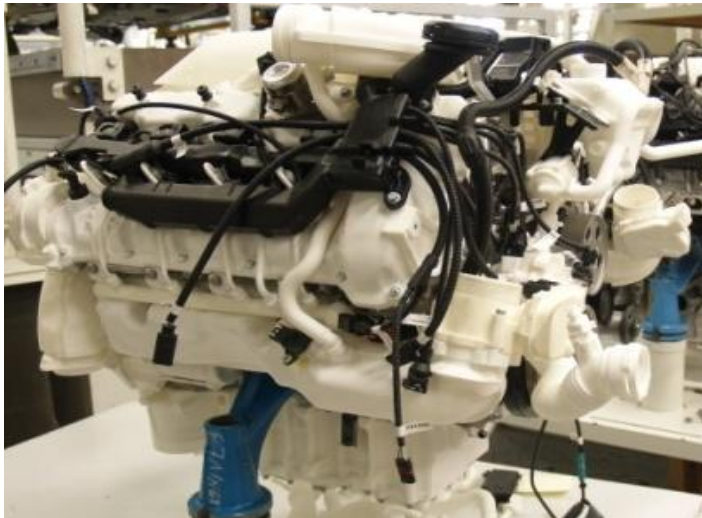
Various motor parts using SLS
