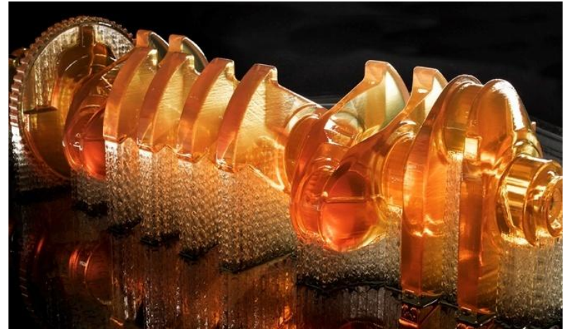
Crankshaft using SLA
