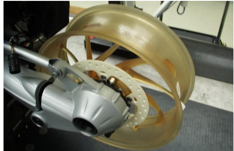
Rear motorcycle wheel using SLA
