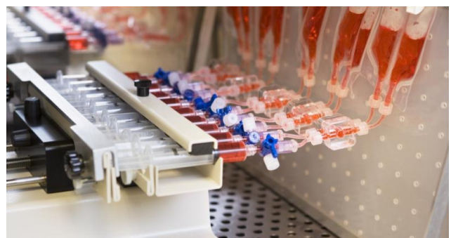
Figure 2: Examples of microfluidics (left, Wyss Institute) and meso-fluidics (right, KIYATEC Inc.) “layered complexity” in vitro systems. Both are perfusion based and incorporate 3D microenvironments and co-culture interactions but differ in scale, manufacturing techniques, cost and throughput.
