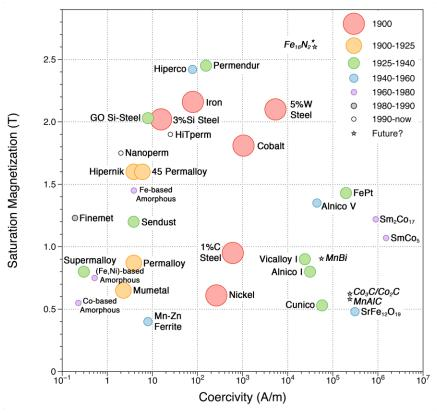
FIGURE 2 Saturation magnetization plotted against coercivity for state-of-the-art magnetic materials. Symbol size and color identify discovery date. Magnetic softness improves to the right and magnetic hardness improves to the left.
