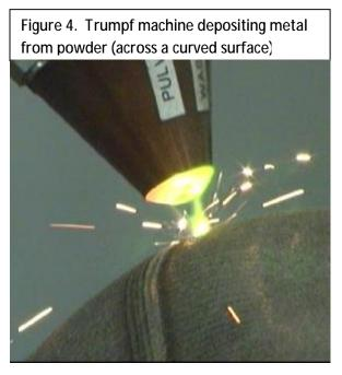
In order to make parts with overhangs, directed energy deposition systems need to either use a 5axis deposition system (so that material can be deposited from any orientation) or a secondary support material. As these systems are typically used to make metal parts or metal/ceramic composite structures, any supports that are used require machining to remove them.
