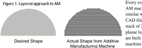
Every existing commercial AM machine works in a similar way. First a 3D CAD file is sliced into a stack of 2-dimensional planar layers. These layers are built by the AM machine and stacked one after the other to build up
