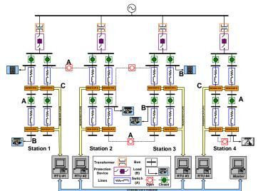
Figure 1: One-line diagram of a multi-phase power distribution system: with control and network inputs (A,B) (e.g. switch, load & faults) and sensed outputs (C)
