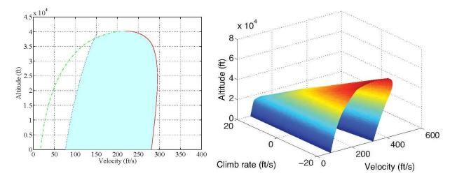
Figure 2: Steady Level (left) and 3-D (right) Traditional Flight Envelope Example [MCC10].
