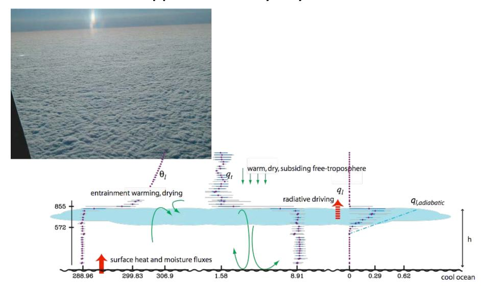
$$\frac{D}{Dt}\langle s \rangle = \overline{w's'}_0 - \overline{w's'}_h - (F_{h_-} - F_0)$$
