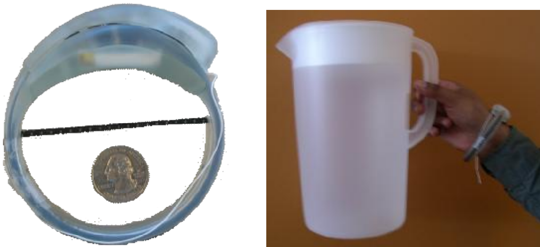
Figure 4 The iBracelet: Close-up (left) with quarter for comparison. In use (right).
