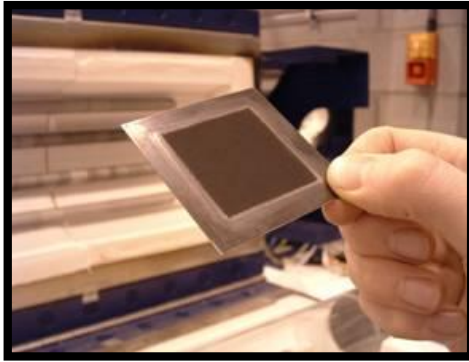
Fig. 2. Example of a metal-supported thin-film solid oxide fuel cell, capable of operation below 600°C. Photo courtesy of Ceres Power, Ltd., reproduced with permission.
