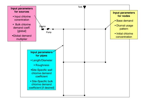
Figure 2. Schematic of model input requirements to simulate chlorine in a distribution system.
