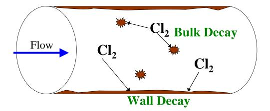
Figure 1. Schematic of Chlorine Decay Reactions in a Distribution System
