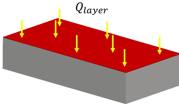
Volumetric heating applied layer-by-layer
