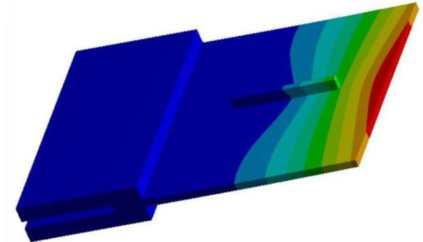
Vertical residual distortion (m) for a five layer line deposit by detailed process simulation (left) and the modified inherent strain method (right)
