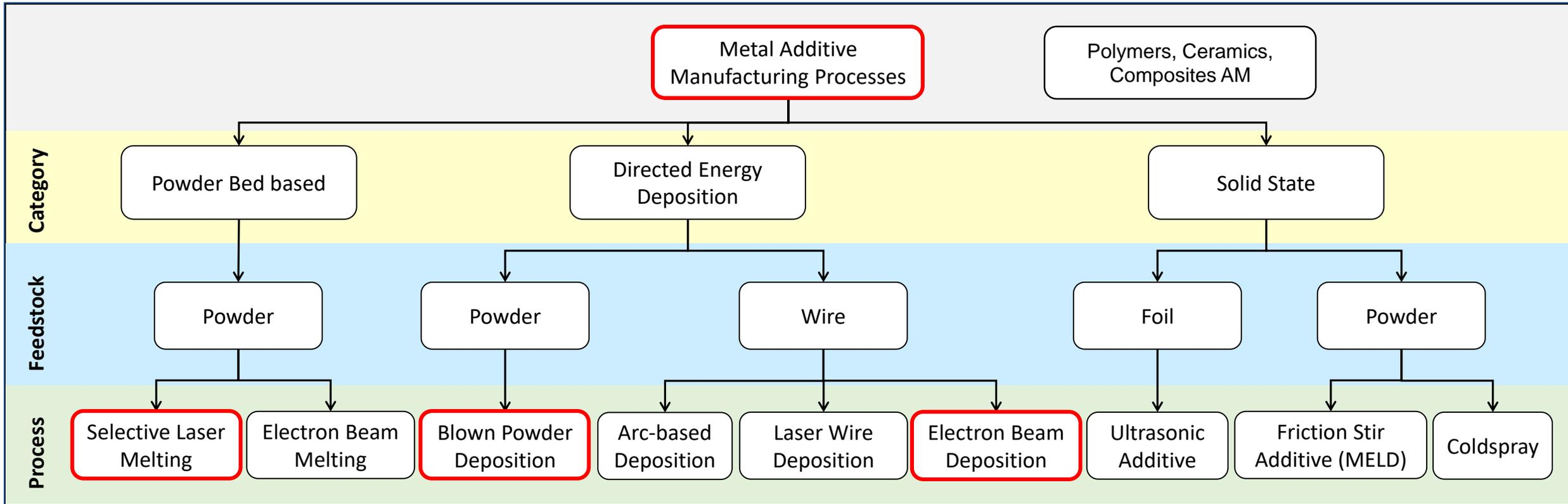
Other metal AM processes are being developed: binder-jet, material extrusion, vat photopolymerization, hybrid methods
