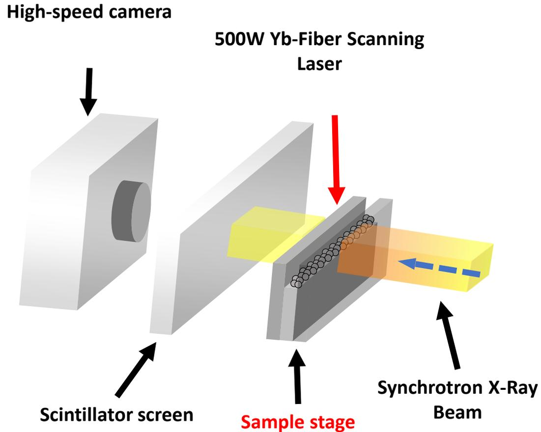
Provides 2D high-speed, in-situ observation of dynamic behavior of powder and melt pool under scanning laser beam
