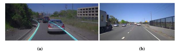
Figure 5: Example of automated labeling of lane lines (a) Hidden lane lines are labeled (b)
