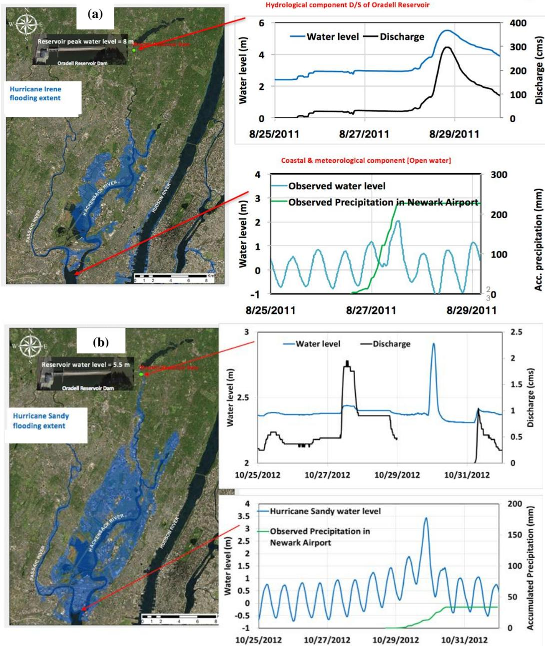
Figure 2. Flooding extent for the combined impact of riverine and tidal components during a) hurricane Irene and b) Sandy showing the observed accumulated precipitation and coastal water levels (including surge) at the Newark Bay.
