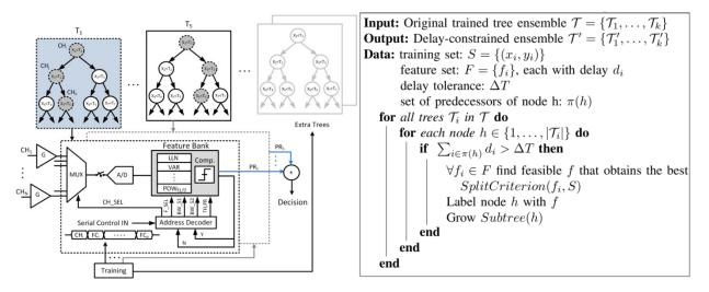
FIGURE 4 Hardware-level architecture for an ensemble of decision tree classifier with primary and supportive trees (left) and a greedy training algorithm to meet the delay constraints (right).
