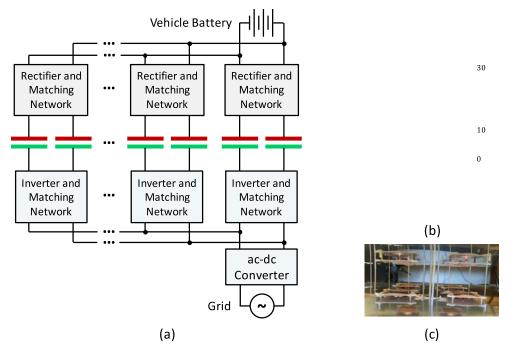
FIGURE 2: Multi-modular near-field phased-array capacitive WPT system: (a) block diagram representation,(b) simulated performance showing fringing field reduction with progressive increase in the number of modules, and (c) photograph of a prototype system.
