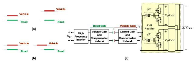
FIGURE 3: Coupling variations and an approach to compensate for these variations: (a) variation in coupling due to different vehicle road clearances, (b) variation in coupling due to change in vehicle position as it drives over the charger, and (c) a capacitive WPT system with an active variable reactance (AVR) rectifier that can provide continuously variable compensation by controlling the voltages V<sub>1</sub> and V<sub>2</sub>.
