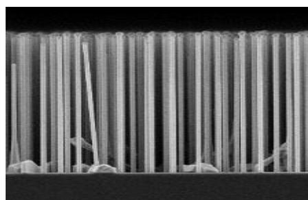
**Fig. 2.** Ordered GaAs nanowires epitaxially grown on Si with lithography-free oxide patterns.
