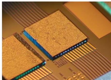
**Fig. 1.** Example of a hybrid integrated circuits including 11 GaInNSbAs-based SOAs mounted on SOI (picture courtesy of Timo Aalto, VTT).
